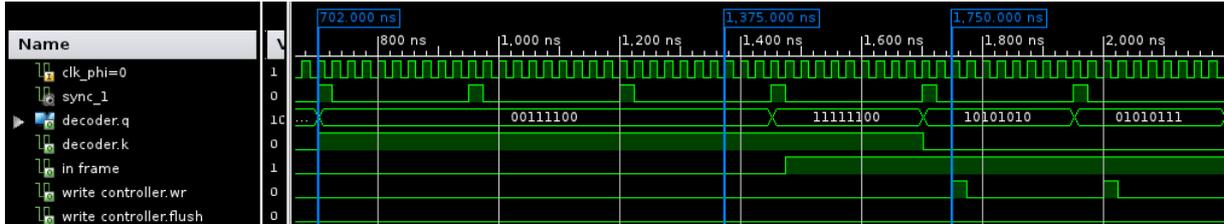
Figure 4.2.: Simulation of the write controller at the beginning of a frame.
