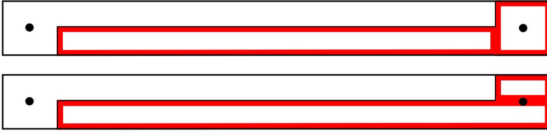
**Figure 5.3.:** A pixel, based on rectangular shapes, is spanned by smaller, red colored rectangles. There can be different possibilities, two of them are shown in this figure for the L shape.
